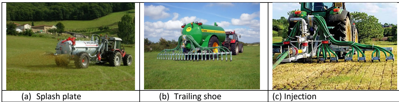
Figure A3. Common slurry application techniques
