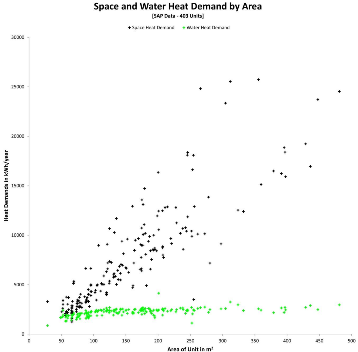
Figure 3: Space and Water Heat Demands plotted by Area of Unit (SAP Data - 403 Units).
