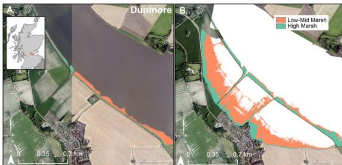
Figure A4.25. Spatial model for Dunmore (A) the extent of present saltmarsh at Dunmore (Haynes, 2016) - inset map of Scotland shows site location; (B) the potential extent of saltmarsh created by managed realignment at this site. High Marsh (green); Low-Mid Marsh (orange).
