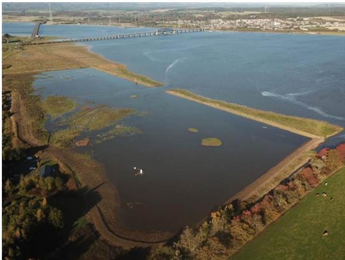
Figure 1. The newly flooded Skinflats, Forth Estuary managed realignment (October 2018), taken shortly before a 6.2m tide (photo credit: J Leonard).
