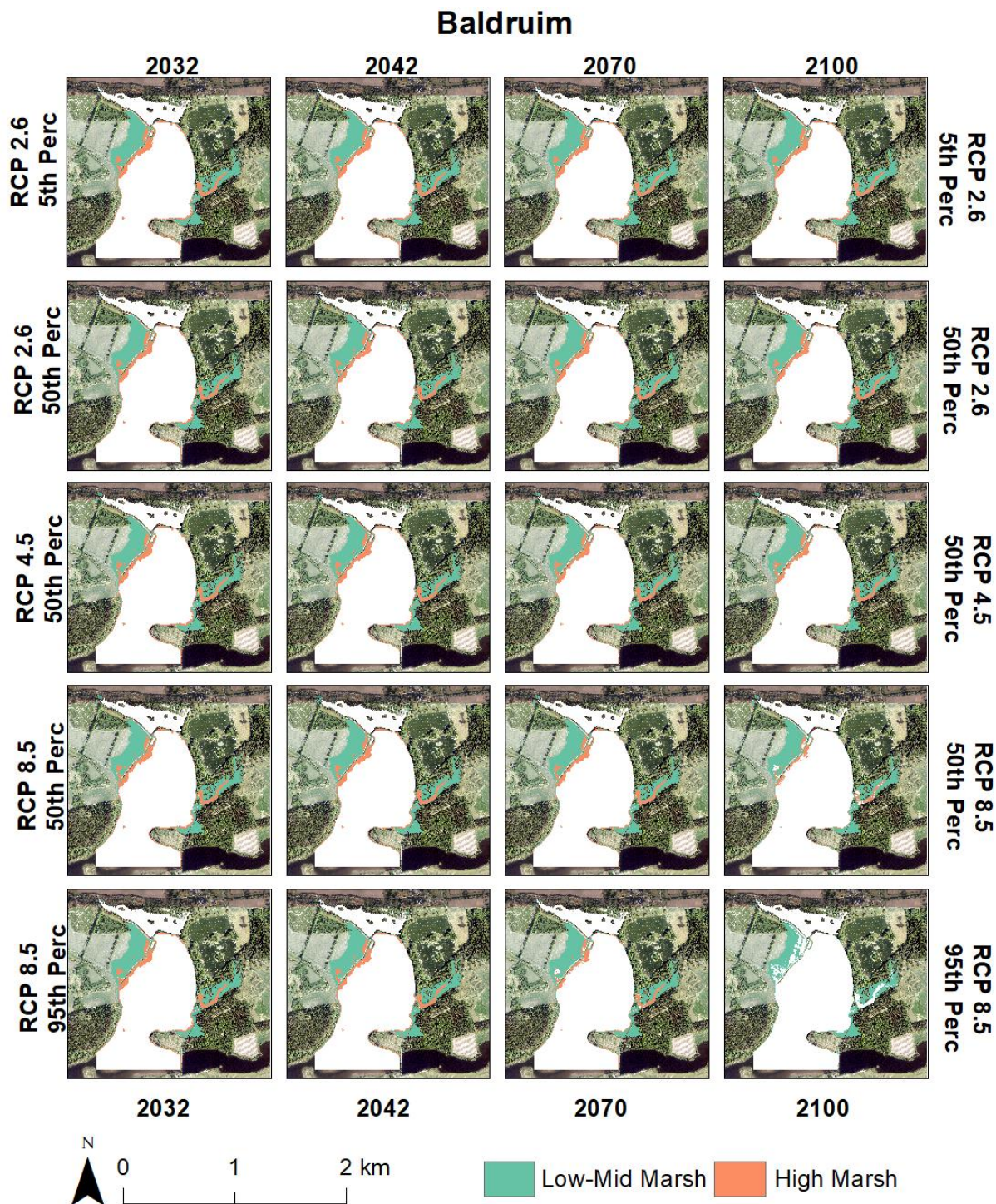
Figure A4.2. Saltmarsh extent following a hypothetical managed realignment at Baldrum, Scotland and including subsequent habitat loss (assuming no landward migration of the coastline nor any vertical accretion of the marsh surface as sea-level rise occurs) from a simple drowning of the saltmarsh surface. Sea-level change projections under different emissions scenarios are shown for the 50 th and 95 th percentiles for RCP 2.6 (low emissions), RCP 4.5 (medium emissions) and RCP 8.5 (high emissions) for 2032, 2045, 2070 and 2100.
