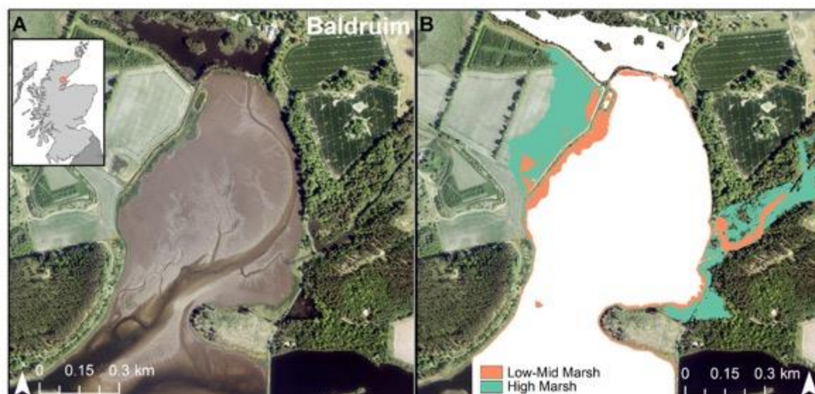
Figure A4.1. Spatial model for Baldrum (A) the extent of present saltmarsh at Baldrum (Haynes, 2016) - inset map of Scotland shows site location; (B) the potential extent of saltmarsh created by managed realignment at this site. High Marsh (green); Low-Mid Marsh (orange).
