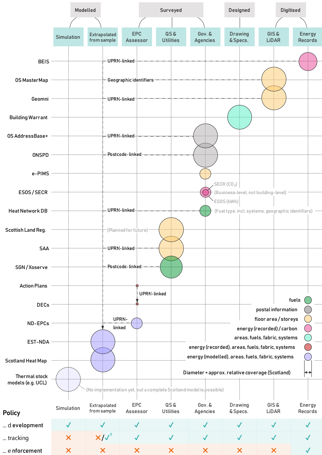
Figure 1: Datasets available in Scotland for ‘policy development’, ‘policy tracking’, and ‘policy enforcement’. Distinct datasets are coloured according to data content (see key), marker size indicates approximate coverage of the data across the Scottish N-D building stock. The datasets are aligned in columns relating to the underlying basis and collection method used, from abstracted models on the left, to verified metered data on the right.
