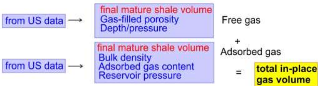
Overview of method used to calculate mature shale gas and shale oil volumes
