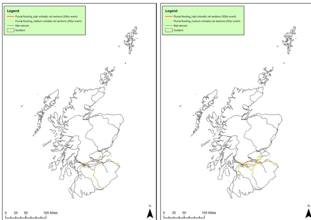
**Figure 2** Sections of the rail network exposed to severe and moderate levels of rail traffic disruption due to fluvial (LH map) and pluvial (RH map) flood hazards (1:200 year event)
