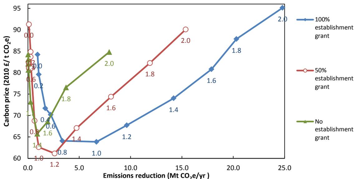
Figure 2. Cost of carbon abatement against annual emission reduction for various subsidy policies, assuming displacement of coal generation. The values below each point show the minimum ROC rates (ROC MWh<sup>-1</sup>) used in that scenario.
