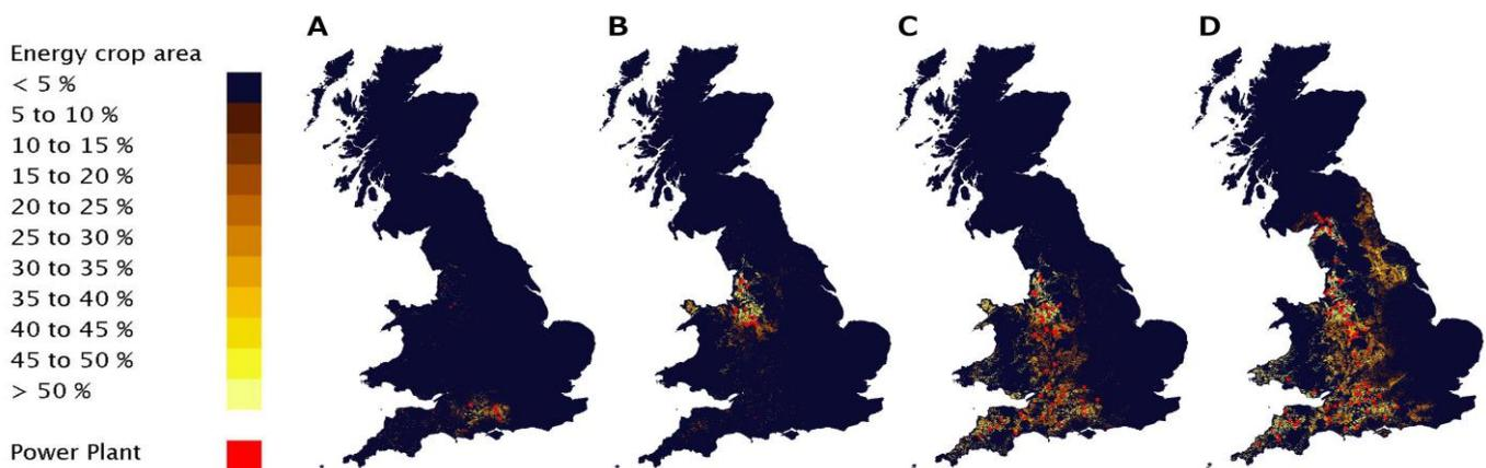
Figure 1. Example distributions of energy crop selection and power plant locations at 2040. A & B from 1.0 ROC  $MWh^{-1}$  minimum ROC rate scenario, C & D showing highest  $CO_2$  equivalent abatement cases from 1.2 & 1.4 ROC  $MWh^{-1}$  minimum ROC rates runs.
